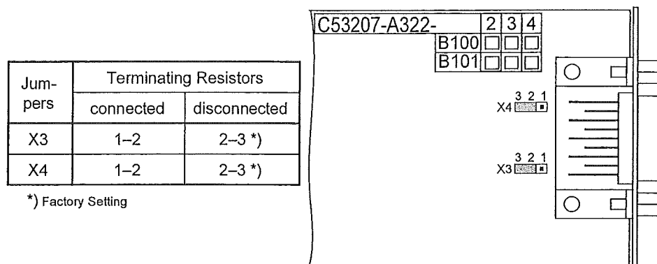
Figure 3-11 Location of the jumpers for the configuration of the termination resistors on the interfaces Profibus DP and DNP3.0
